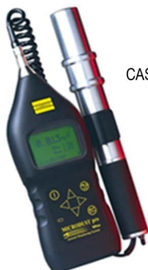
Photo 3.1: Digital CASELLA microdust and 6-gas MX6 iBrid™ meters to be used measure air quality
