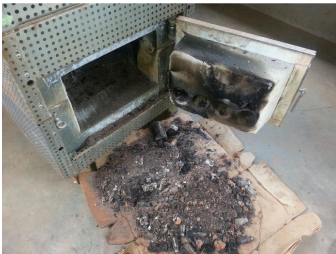
Figure 3: Incomplete combustion as exhibited in the ash content and the soot on the incinerator door
