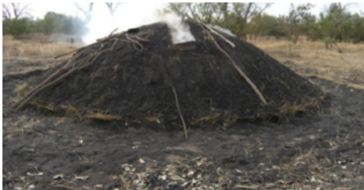
Figure 3. Earth-mound method of charcoal production
