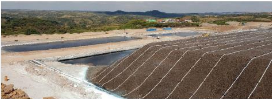
Figure 4: Heap leach under operation with drip irrigation spreading desorption/leach solution across the heap in the foreground, and solution collection ponds in the background
