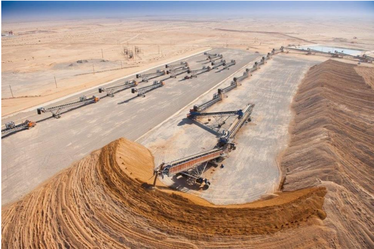
Figure 33: Stacking ore on liner for heap leaching http://miningmirror.co.za/2018/07/11/heap-leaching-a-stack-of-gold/
