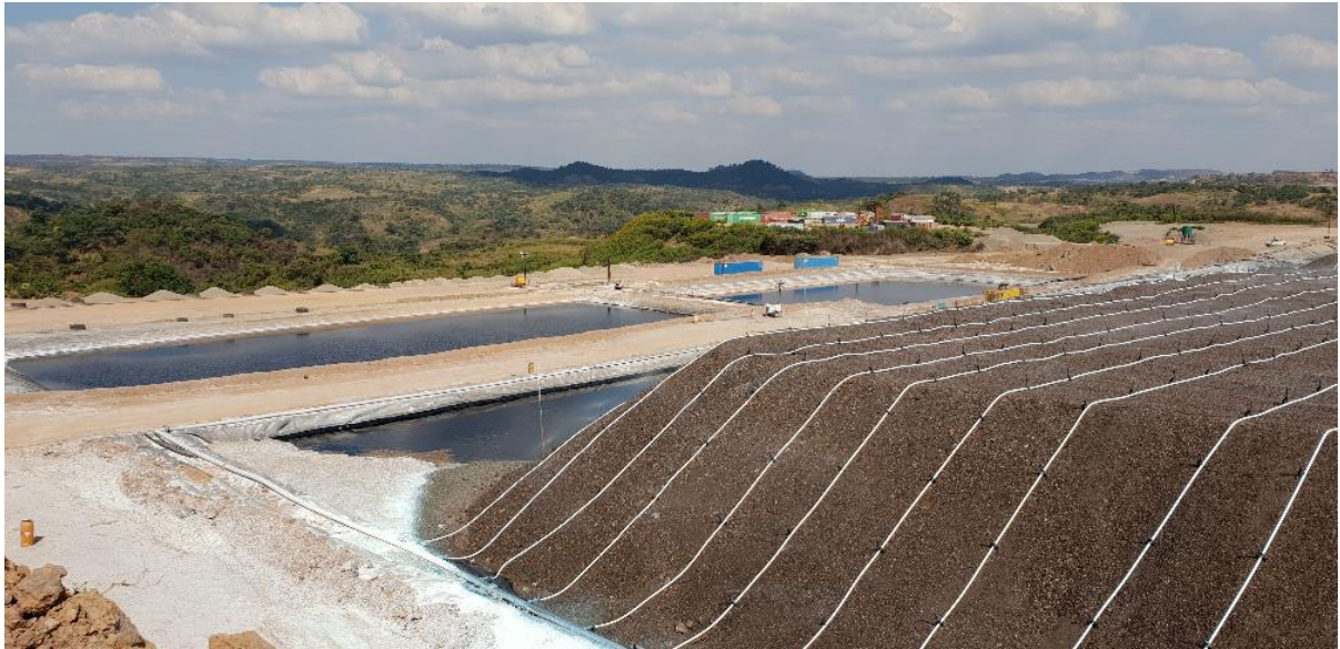
Figure 34: Application of leach liquor to heap leach pads
