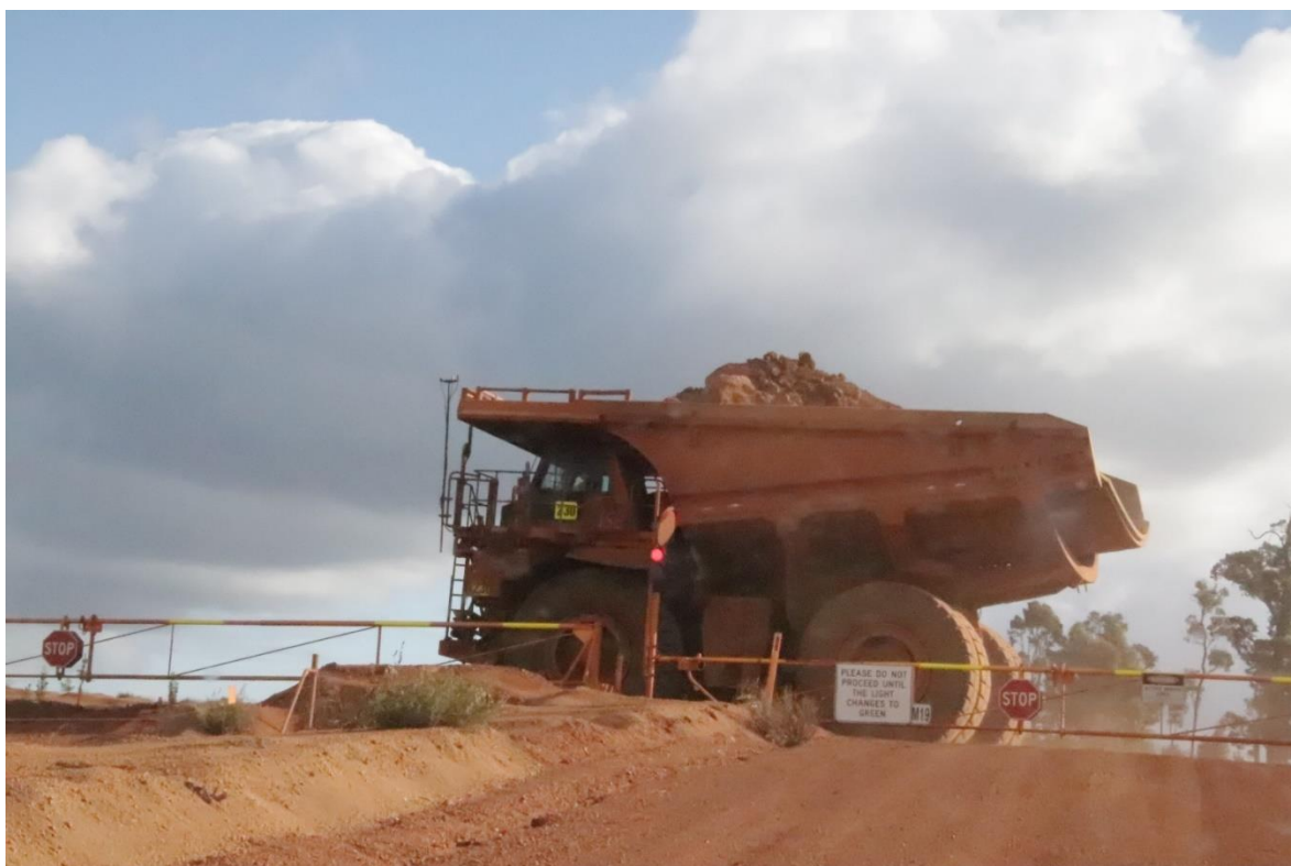
Figure 167: Controlled bauxite haul road crossing in Australia similar to what is planned for Makuutu.
