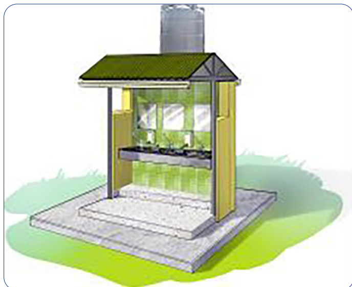
Figure 2.4.4: Sample design of the Millions of Clean Hands (MoCH) hand washing station
