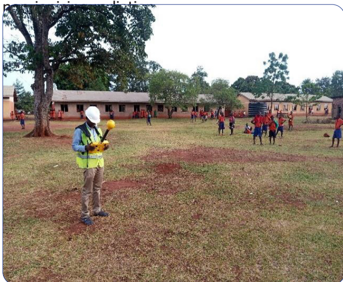
Figure 2.3.3: Measurement of RF exposure levels at the base of a telecommunication tower in Kamuli District. Source: AEC 2021
